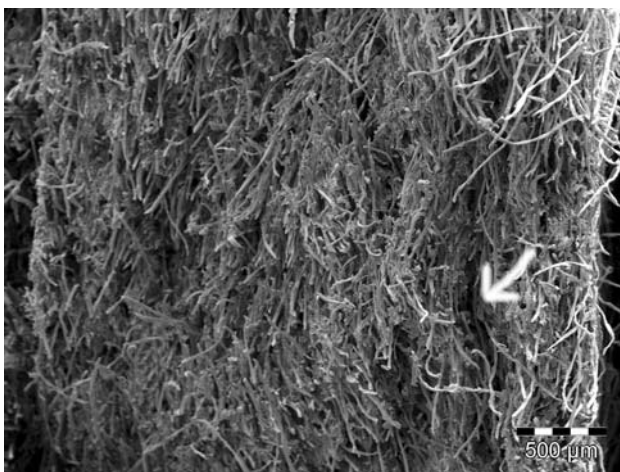
Fig. 7 SEM photograph of a fractured surface of a cotton/PLA + lignin composite (overview)
